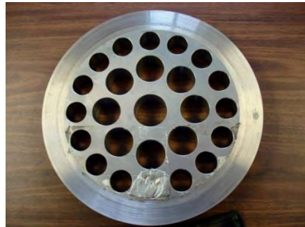
12-inch, 4-Path Meter - 1 Hole Blocked Results
