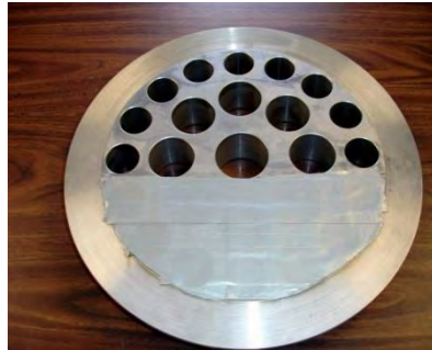
12-inch, 4-Path Meter - 40% Blocked Results
